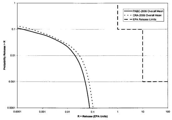
Figure 3-13: PABC-2009 and CRA-2009 Overall Mean CCDFs for Normalized Spallings Releases
