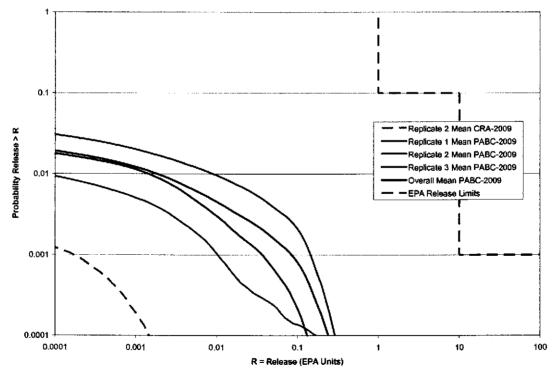
Figure 3-27: PABC-2009 and CRA-2009 Replicate Mean CCDFs for Normalized Culebra Transport Releases
