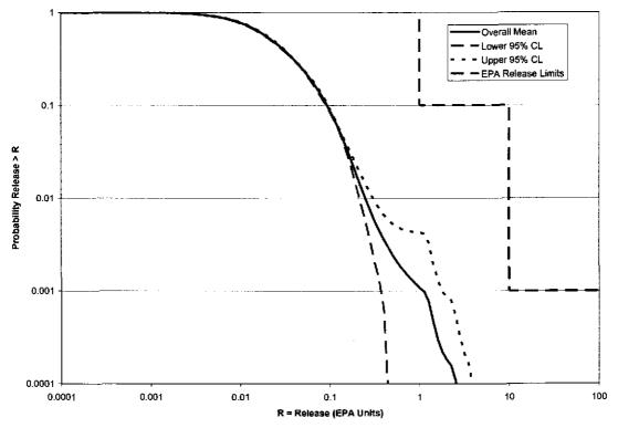
Figure 3-33: PABC-2009 Confidence Limits on Overall Mean for Total Normalized Releases
