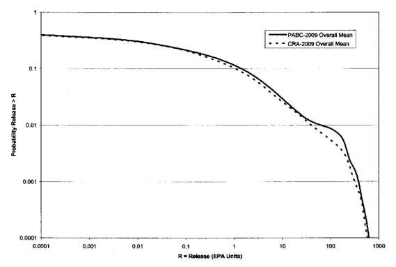
Figure 3-28: PABC-2009 and CRA-2009 Overall Mean CCDFs for Transport Releases to the Culebra
