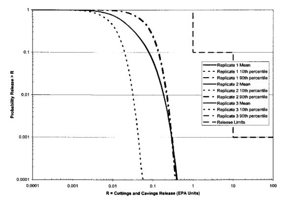
Figure 3-4: PABC-2009 Mean and Quantile CCDFs for Cuttings and Cavings Normalized Releases, Replicates 1-3
