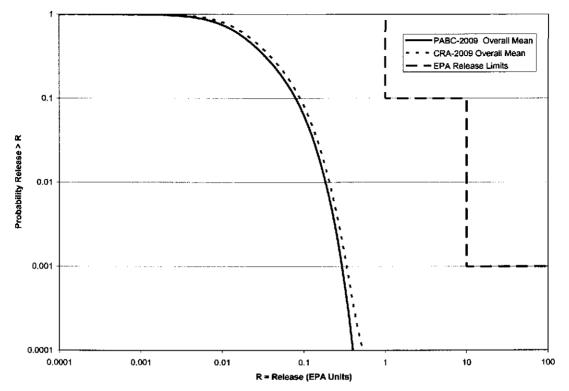
Figure 3-6: PABC-2009 and CRA-2009 Overall Mean CCDFs for Normalized Cuttings and Cavings Releases
