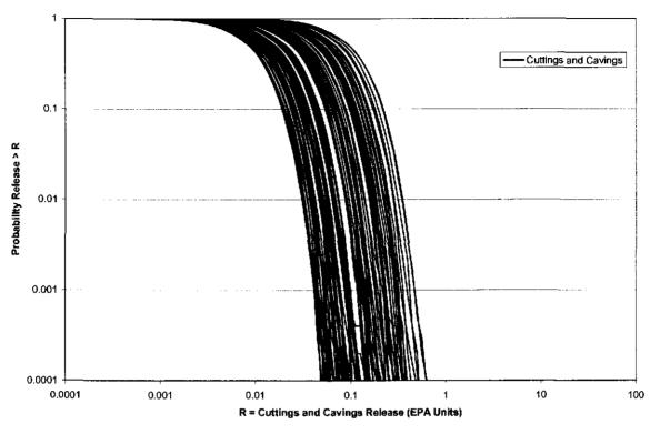
Figure 3-2: PABC-2009 Replicate 2 Cuttings and Cavings Normalized Releases
