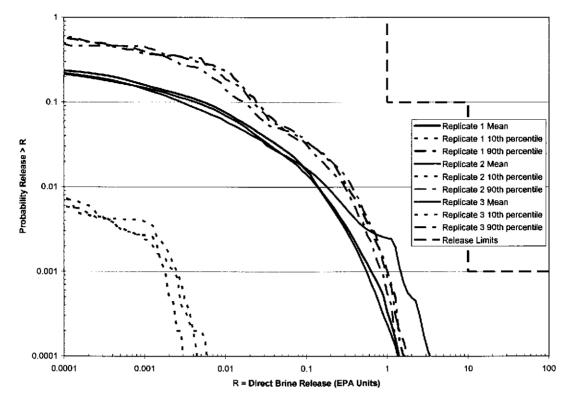
Figure 3-18: PABC-2009 Mean and Quantile CCDFs for Normalized Direct Brine Releases, Replicates 1-3
