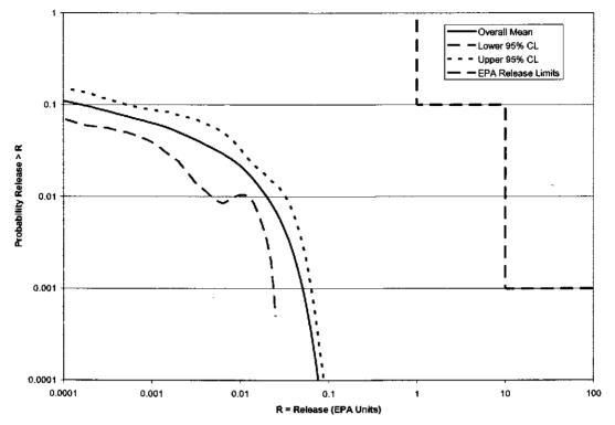
Figure 3-12: PABC-2009 Confidence Limits on Overall Mean for Spallings Normalized Releases
