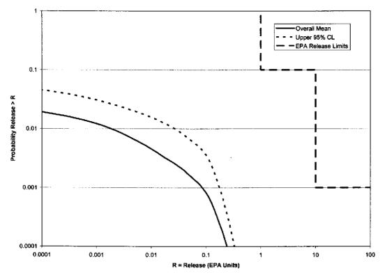
Figure 3-26: PABC-2009 Confidence Limits on Overall Mean for Normalized Culebra Transport Releases
