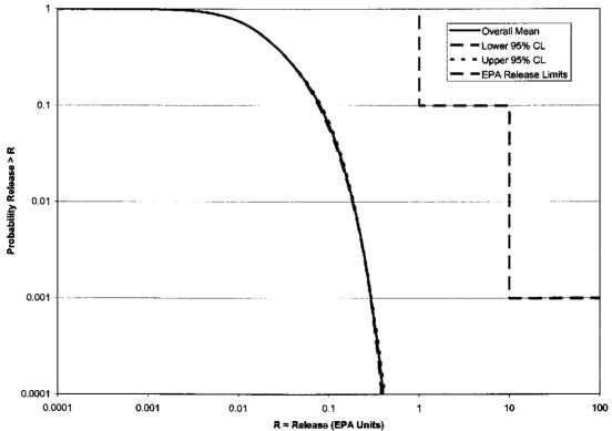
Figure 3-5: PABC-2009 Confidence Limits on Overall Mean for Cuttings and Cavings Normalized Releases
